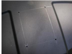
**Step 2:** Use your cut-off gutter spout as a template to draw an opening on your barrel lid. Use a utility knife to cut along the lines, creating an entry point for the gutter spout.
