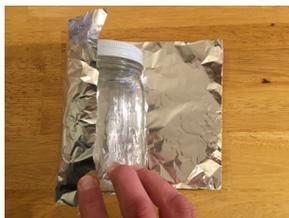
**Step 1:** Estimate the amount of aluminum foil (*height and width*) needed to line the inside of the jar—wrapping the aluminum foil around the outside and cutting to length works well.
