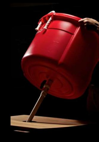
2. Place the 2" PVC section of the stand pipe (with filters attached) over the smaller PVC section of the stand pipe that is attached in the center of the tub. It should rest on the bottom of the tub.
