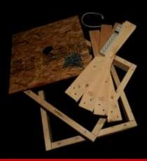
•Two square frames – top and bottom •Four legs, one with a power strip attached •Plywood top with hole in center •16 carriage bolts, 16 washers, & 16 wing nuts
