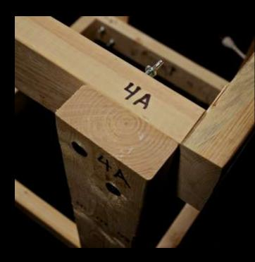
2. Insert carriage bolts, then place washer and tighten wing nut.
